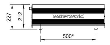
\*Mounting feet adjustable along T-slot
