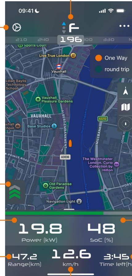
**Throttle position & compass**– Displays the current heading and the position of the throttle
