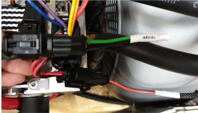
2. If the green/black cable is not connected, then the "cut-off" voltage, the minimum voltage at which the controller stops working, is 42 Volts, and the warning on the display appears at 44 Volts.
