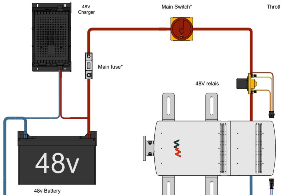
Ensure that the main power switch, once the system is installed, is always in the OFF position ("0" or "off") during work on the components and when disconnecting and connecting power cables.
