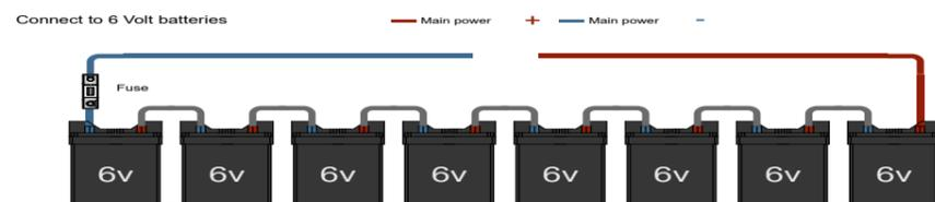
**WARNING! Wait with connecting the batteries to the rest of the system until everything is connected and has been tested for any short circuits.**
