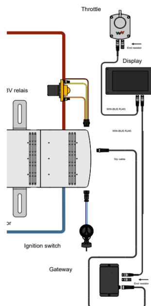
**Starting from 2022 with software version  $\geq$  1.31, only follow steps 1, 2, and 5. Place an end resistor in the remaining contacts.**
