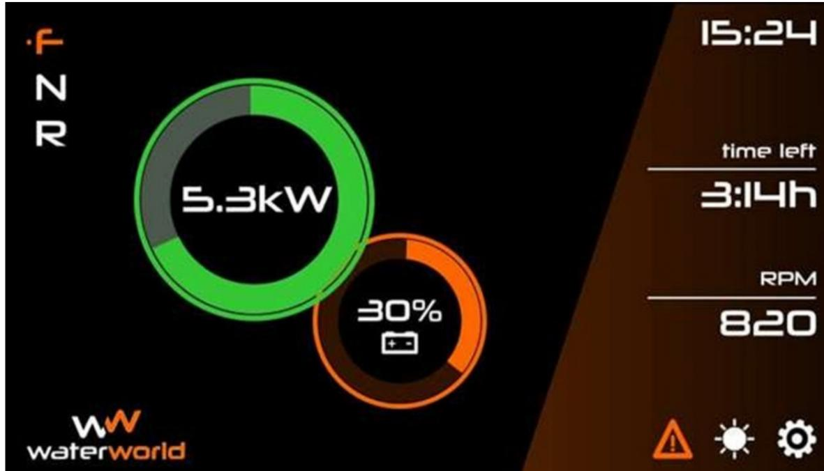
The letters **F (Forward)**, **N (Neutral)**, and **R (Reverse)** in the top left corner of the screen indicate whether your throttle lever is in forward, neutral, or reverse.
